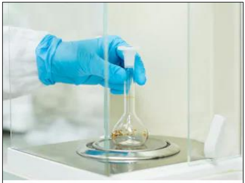
Calibration of one-mark volumetric flask
